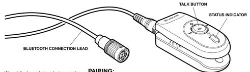
When fully charged, the adapter provides a minimum of eight hours talk time and three hundred hours standby time.
