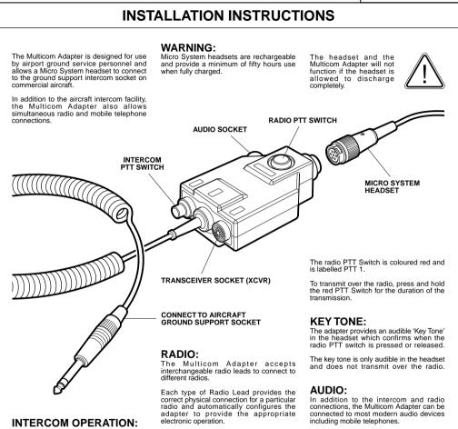
To establish intercom communication with an aircraft, connect the Multicom Adapter jack plug to the ground support intercom socket on the aircraft.
