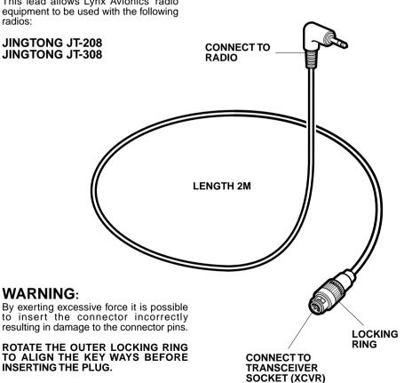
ROTATE THE OUTER LOCKING RING INSERTING THE PLUG.
